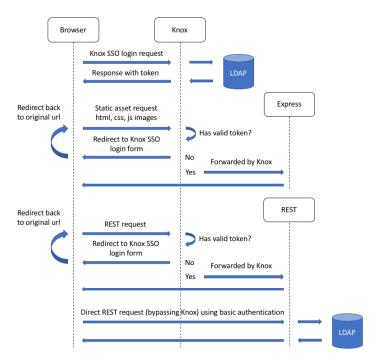
Note how the flow diagrams for Static asset requests and Rest requests (through Knox) are identical.
