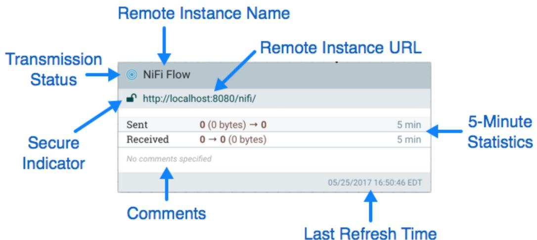
The image above shows the different elements that make up a Remote Process Group. Here, we provide an explanation of the icons and details about the information provided.
