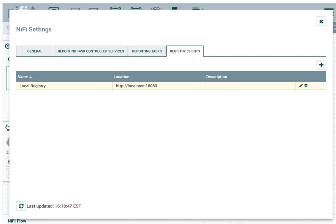
Versioned flows are stored and organized in registry buckets. Bucket Policies and Special Privileges configured by the registry administrator determine which buckets a user can import versioned flows from and which buckets a user can save versioned flows to. Information on Bucket Policies and Special Privileges can be found in the NiFi Registry User Guide (<https://nifi.apache.org/docs/nifi-registry-docs/html/user-guide.html>).
