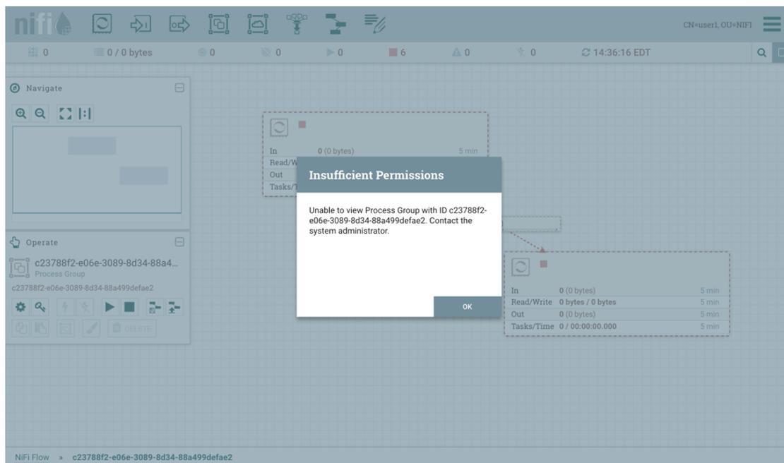
If a user has access to View a process group but does not have access to Modify the process group, the variables can be viewed but not modified.
