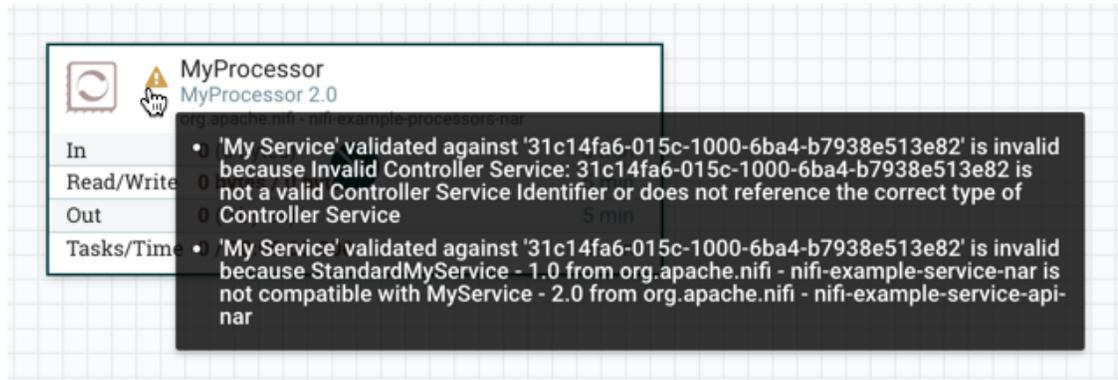
and an error message will be displayed in the processor's controller service configuration since the service is no longer valid:
