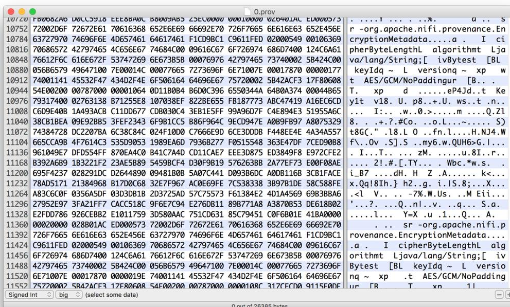
On record read, the process is reversed. The encryption metadata is parsed and used to decrypt the serialized bytes, which are then deserialized into a `ProvenanceEventRecord` object. The delegation to the normal schema record writer/reader allows for "random-access" (i.e. immediate seek without decryption of unnecessary records).
