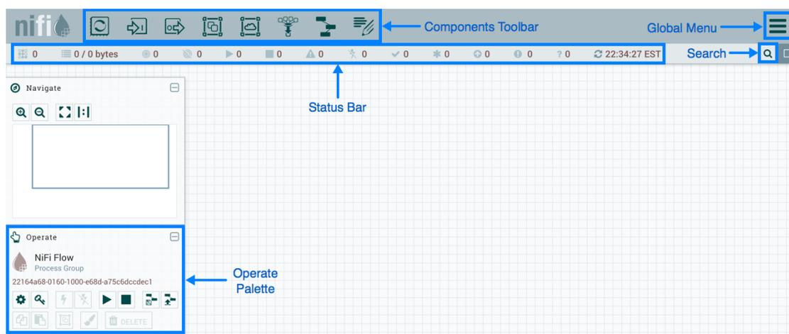
The Components Toolbar runs across the top left portion of your screen. It consists of the components you can drag onto the canvas to build your dataflow. Each component is described in more detail in [Building a Dataflow](#).
