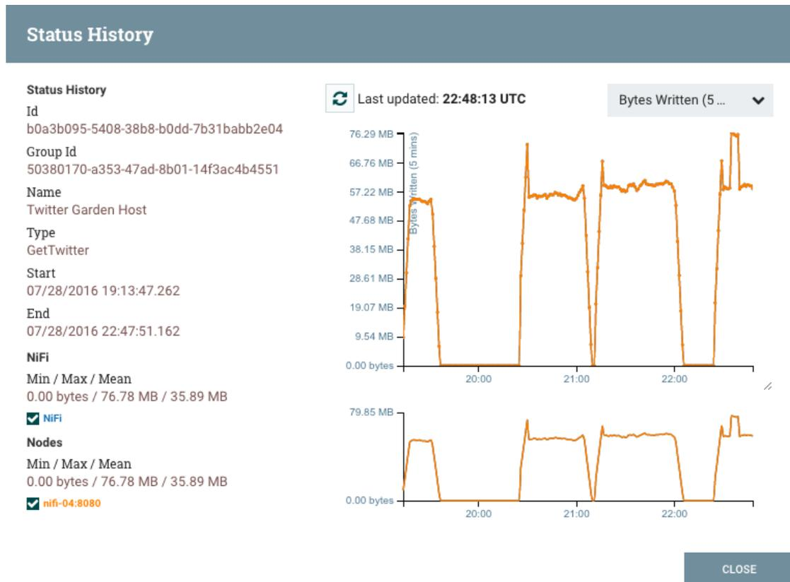
The left-hand side of the dialog provides information about the component that the stats are for, as well as a textual representation of the statistics being graphed. The following information is provided on the left-hand side:
