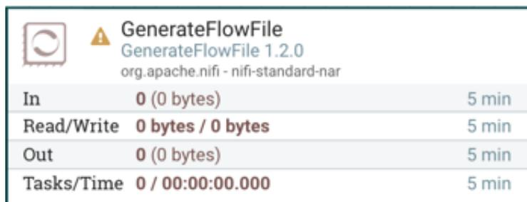
In this case, hovering over the indicator icon with the mouse will provide a tooltip showing all of the validation errors for the Processor. Once all of the validation errors have been addressed, the status indicator will change to a Stop icon, indicating that the Processor is valid and ready to be started but currently is not running:
