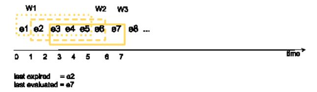
If the system crashes, tuples e1 to e8 are replayed, assuming that the ack for e1 and e2 did not reach the acker. Tuples w1, w2 and w3 will be reevaluated.
