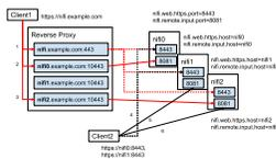
1. Client1 initiates Site-to-Site protocol, the request is routed to one of upstream NiFi nodes. The NiFi node computes Site-to-Site port for RAW. By the routing rule 'example1' in nifi.properties shown below, port 10443 is returned.
