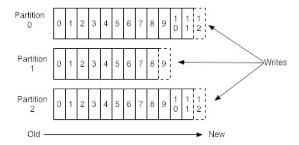
Kafka appends new messages to a partition in an ordered, immutable sequence. Each message in a topic is assigned a sequential number that uniquely identifies the message within a partition. This number is called an offset, and is represented in the diagram by numbers within each cell (such as 0 through 12 in partition 0).
