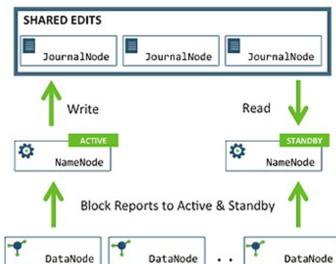
It is vital for the correct operation of an HA cluster that only one of the NameNodes should be active at a time. Failure to do so, would cause the namespace state to quickly diverge between the two NameNode machines thus causing potential data loss. This situation is called a *split-brain scenario*.
