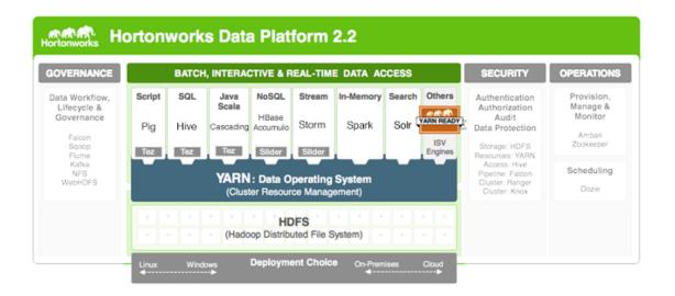
The core components of HDP are YARN and the Hadoop Distributed File System (HDFS).
