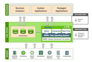
**HDFS** (storage) works closely with MapReduce (data processing) to provide scalable, fault-tolerant, cost-efficient storage for big data. By distributing storage and computation across many servers, the combined storage resource can grow with demand while remaining economical at every size.
