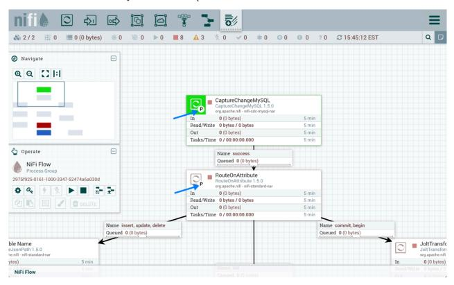
To quickly identify 'Primary Node' processors, the "P" icon is also shown in the Processors tab on the Summary page:
