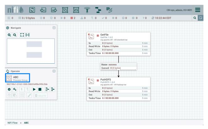
GetFile processor is a restricted component that requires 'write filesystem' and 'read filesystem' permissions:
