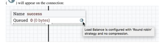
Hovering over the icon will display the connection's load balance strategy and compression configuration. The icon in this state also indicates that all data in the connection has been distributed across the cluster.
