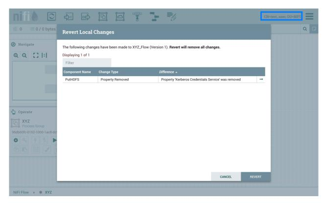
the revert is unsuccessful because test\_user does not have the 'access keytab' permissions required by the KeytabCredentialService controller service:
