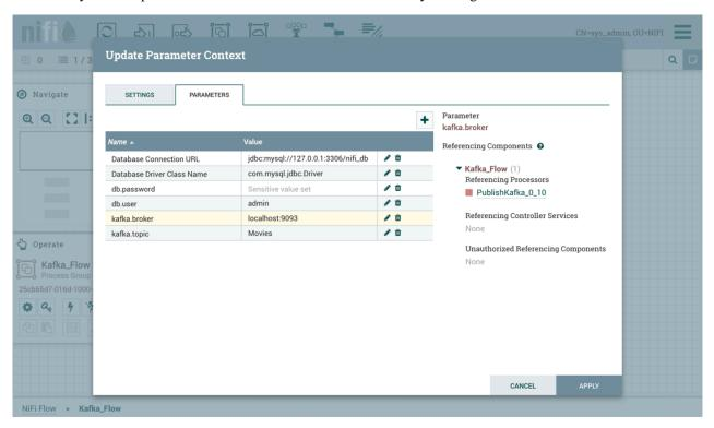
To complete the process, select "Apply" from the Parameter Context window. The following operations are performed to validate all components that reference the added or modified parameters: Stopping/Restarting affected Processors, Disabling/Re-enabling affected Controller Services, Updating Parameter Context.
