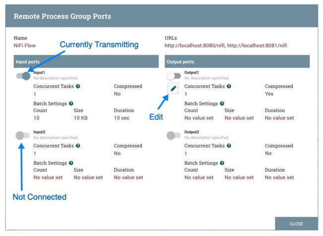
The on/off toggle switch provides a mechanism to enable and disable transmission for each port in the Remote Process Group independently. Those ports that are connected but are not currently transmitting can be configured by
