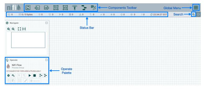
The Components Toolbar runs across the top left portion of your screen. It consists of the components you can drag onto the canvas to build your dataflow. Each component is described in more detail in 9243981bc34267c7ff4fd1eb910e2420631d8727.html#building-dataflow.
