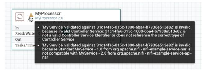
and an error message will be displayed in the processor's controller service configuration since the service is no longer valid:
