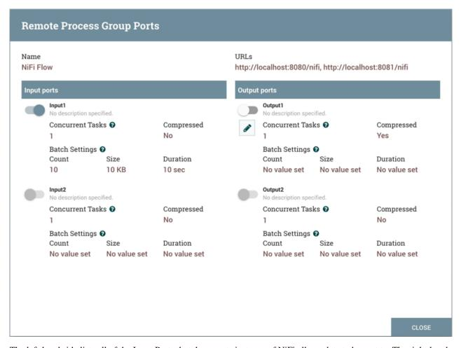
The left-hand side lists all of the Input Ports that the remote instance of NiFi allows data to be sent to. The right-hand side lists all of the Output Ports from which this instance is able to pull data. If the remote instance is using secure communications (the URL of the NiFi instance begins with https://, rather than http://), any ports that the remote instance has not made available to this instance will not be shown.
