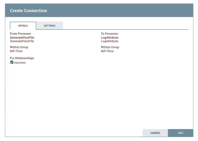
Additionally, this tab provides the ability to choose which Relationships should be included in this Connection. At least one Relationship must be selected. If only one Relationship is available, it is automatically selected.
