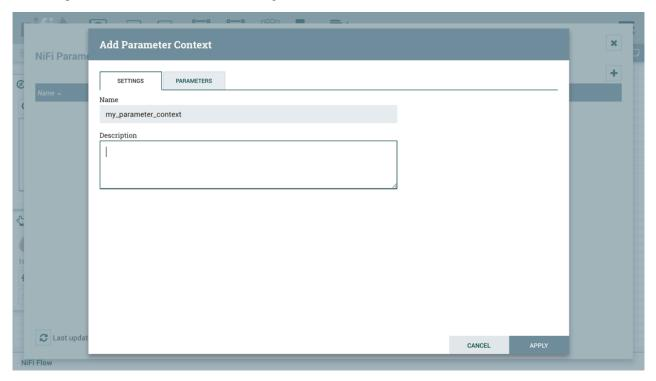
On the "Settings" tab, add a name for the Parameter Context and a description if desired. Select "Apply" to save the Parameter Context or select the "Parameters" tab to add parameters to the context.
