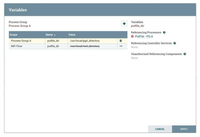
A variable can only be modified for the process group it was created in, which is listed at the top of the Variables window. To modify a variable defined in a different process group, select the "arrow" icon in that variable's row:
