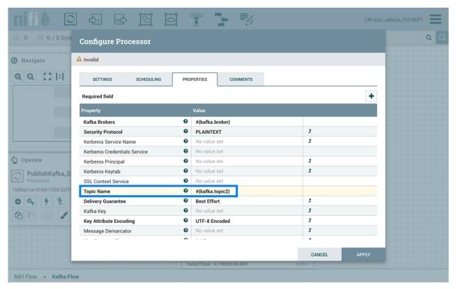
Properties values that are selectable can also reference parameters. In addition to applying the "Convert to Parameter" method described earlier, the option "Reference parameter.." is available in the value drop-down menu.
