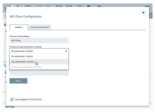
Select "Apply" to save the configuration changes. The Process Group context menu now includes a "Parameters" option which allows quick access to the Update Parameter Context window for the assigned Parameter Context.
