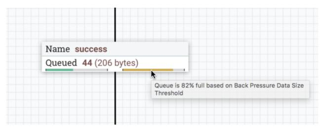
When the queue is completely full, the Connection is highlighted in red.
