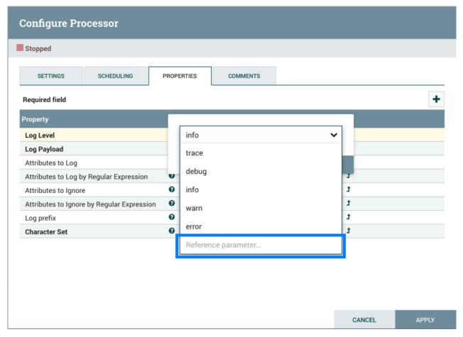
Selecting "Reference parameter..." will display a drop-down list of available parameters, determined by the parameter context assigned to the component's process group and the user's access policies.
