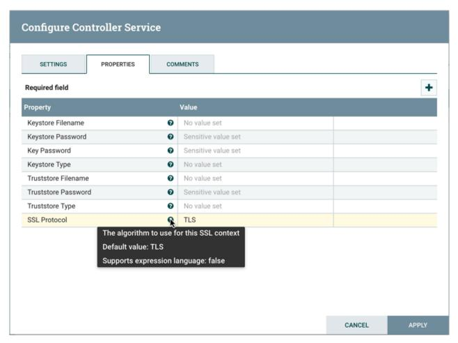
The Comments tab is just an open-text field, where the DFM may include comments about the service. After configuring a Controller Service, click "Apply" to save the configuration and close the window, or click "Cancel" to discard the changes and close the window.
