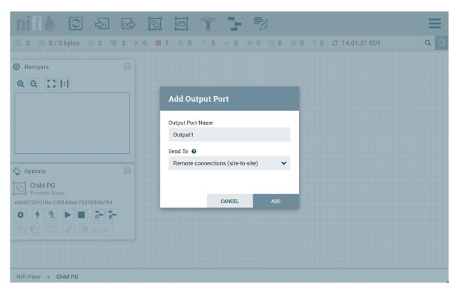
In addition to other instances of NiFi, some other applications may use a Site-to-Site client in order to push data to or receive data from a NiFi instance. For example, NiFi provides an Apache Storm spout and an Apache Spark Receiver that are able to pull data from NiFi's Output Ports for Site-to-Site connections.
