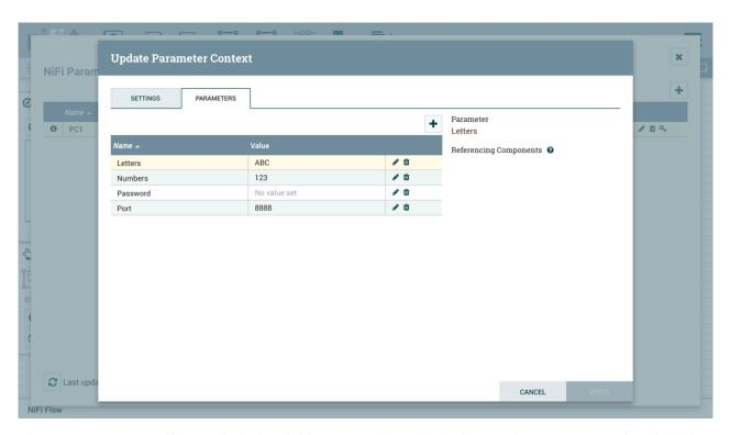
The "Letters" parameter did not exist in the NiFi instance and was added. The "Numbers" parameter existed in both the versioned flow and NiFi instance with identical values, so no changes were made. "Password" is a sensitive Parameter missing from the NiFi instance, so it was added but with no value. "Port" existed in the NiFi instance with a different value than the versioned flow, so its value remained unchanged.
