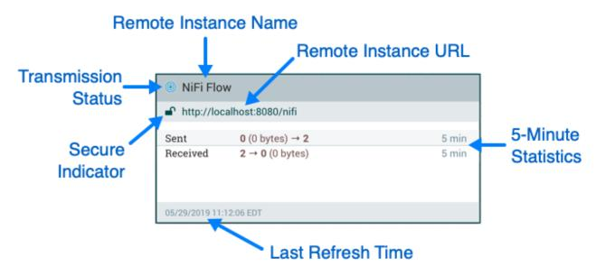
The image above shows the different elements that make up a Remote Process Group. Here, we provide an explanation of the icons and details about the information provided.
