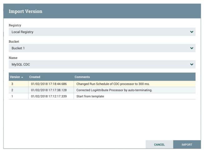
Connected registries will appear as options in the Registry drop-down menu. For the chosen Registry, buckets the user has access to will appear as options in the Bucket drop-down menu. The names of the flows in the chosen bucket will appear as options in the Name drop-down menu. Select the desired version of the flow to import and select "Import" for the dataflow to be placed on the canvas.
