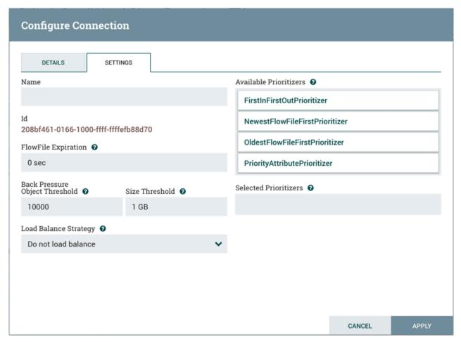
The Connection name is optional. If not specified, the name shown for the Connection will be names of the Relationships that are active for the Connection.
