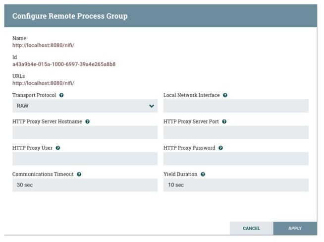
By default, it is set to RAW which uses raw socket communication using a dedicated port. HTTP transport protocol is especially useful if the remote NiFi instance is in a restricted network that only allow access through HTTP(S) protocol or only accessible from a specific HTTP Proxy server. For accessing through a HTTP Proxy Server, BASIC and DIGEST authentication are supported.
