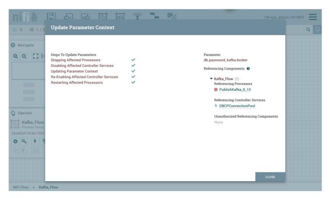
The Referencing Components section now lists an aggregation of all the components referenced by the set of parameters added/edited/deleted, organized by process group.
