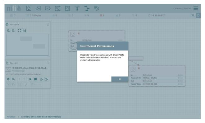
If a user has access to View a process group but does not have access to Modify the process group, the variables can be viewed but not modified.
