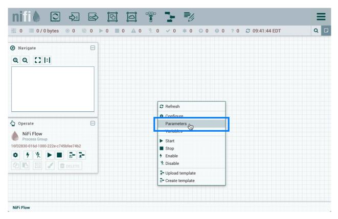
If the Parameter Context for a Process Group is changed, all components that reference any Parameters in that Process Group will be stopped, validated, and restarted assuming the components were previously running and are still valid.
