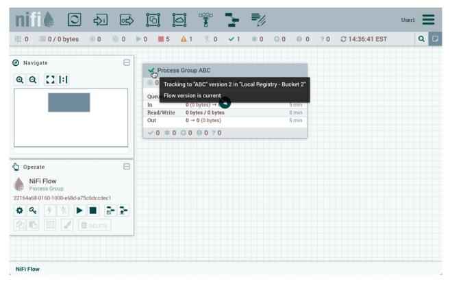
In the example shown, the versioned flow is upgraded from an older to the newer latest version. However, a versioned flow can also be rollbacked to an older version.
