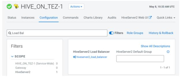
**2.** Set the value, using the following format: <hostname>:<port number>. For example, hs2load balancer.example.com:10015.
