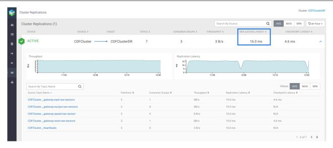
In the image, you can see the average replication latency for the CDFCluster to CDFClusterDR replication is 16.0 milliseconds. You can fetch the maximum or minimum replication latency for the replication by clicking the MAX or MIN button located above the cluster replication.
