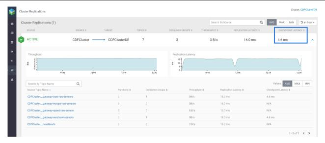
In the image, you can see the average checkpoint latency for the CDFCluster to CDFClusterDR replication is 4.6 milliseconds. You can fetch the maximum or minimum replication latency for the replication by clicking the MAX or MIN button located above the cluster replication.
