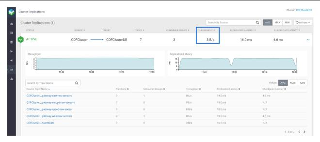
In the image, you can see the average throughput for the CDFCluster to CDFClusterDR replication is 3 bytes per second. You can fetch the maximum or minimum throughput for the replication by clicking the MAX or MIN button located above the cluster replication.
