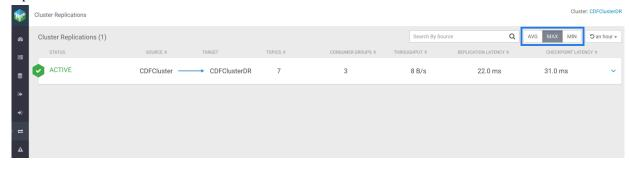
Topic Level. Click the AVG, MAX, or MIN buttons, as shown in the following image, to fetch average, maximum, or minimum values of throughput, replication latency, and checkpoint latency for topics.
