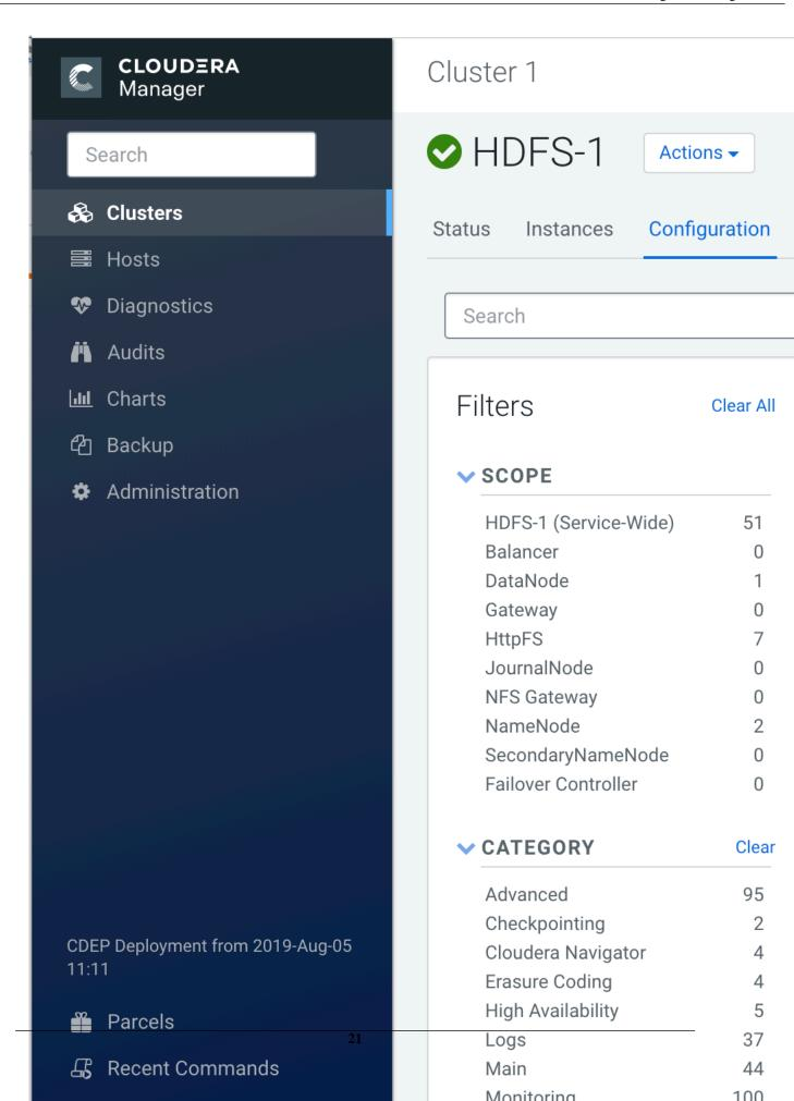
The Kerberos principal short name for the HDFS service,"hdfs", is the one that is involved the second communication channel (RPS to components) for getting metadata from HDFS (such as HDFS folders) across. The settings on the HDFS configuration must match those set in Ranger (by selecting Access > Manager > Resource Based Policies, then selecting the Edit icon for the HDFS service:
