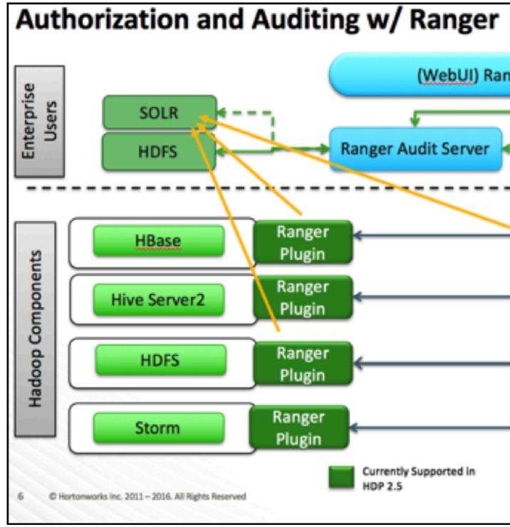
When a Ranger plugin for a component (such as HBase or HDFS) is activated, Ranger is in full control of any access. There is two-way communication between the Ranger plugin and the Ranger (Admin) Policy Server (RPS):
