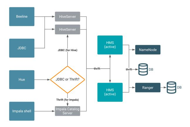
HMS connects directly to Ranger and the NameNode (HDFS), and so does HiveServer, but this is not shown in the diagram for simplicity. One or more HMS instances on the backend can talk to other services, such as Ranger.
