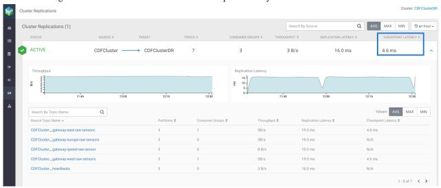
In the image, you can see the average checkpoint latency for the CDFCluster to CDFClusterDR replication is 4.6 milliseconds. You can fetch the maximum or minimum replication latency for the replication by clicking the MAX or MIN button located above the cluster replication.
