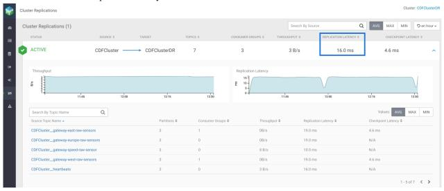
In the image, you can see the average replication latency for the CDFCluster to CDFClusterDR replication is 16.0 milliseconds. You can fetch the maximum or minimum replication latency for the replication by clicking the MAX or MIN button located above the cluster replication.
