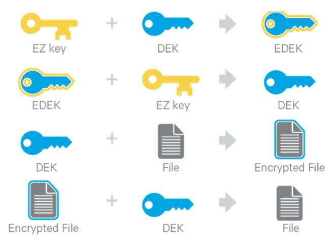
EDEKs are stored persistently on the NameNode as part of each file's metadata, using HDFS extended attributes. EDEKs can be safely stored and handled by the NameNode because the hdfs user does not have access to the EDEK's encryption keys (EZ keys). Even if HDFS is compromised (for example, by gaining unauthorized access to a superuser account), a malicious user only gains access to the encrypted text and EDEKs. EZ keys are controlled by a separate set of permissions on the KMS and the keystore.
