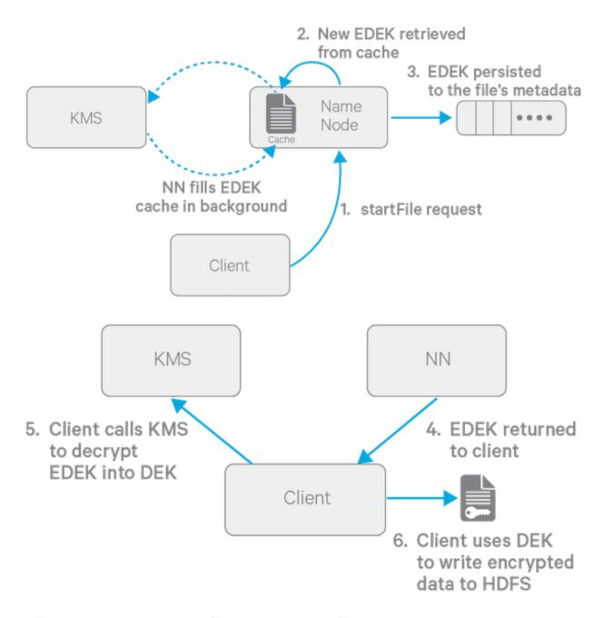
The diagram above depicts the process of writing a new encrypted file. Note that the EDEK cache on the NameNode is populated in the background. Since it is the responsibility of KMS to create EDEKs, using a cache avoids having to call the KMS for each create request. The client can request new EDEKs directly from the NameNode.
