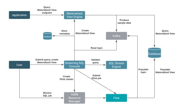
The primary point of user interaction for SQL Stream Builder is the Console component. When you submit a query using the Streaming SQL Console, a Flink job is automatically created in the background on the cluster. SSB also requires a Kafka service on the same cluster. This mandatory Kafka service is used to automatically populate topics for the websocket output. The websocket output is needed for sampling data to the Console, and when no table is added to output the results of the SQL query.
