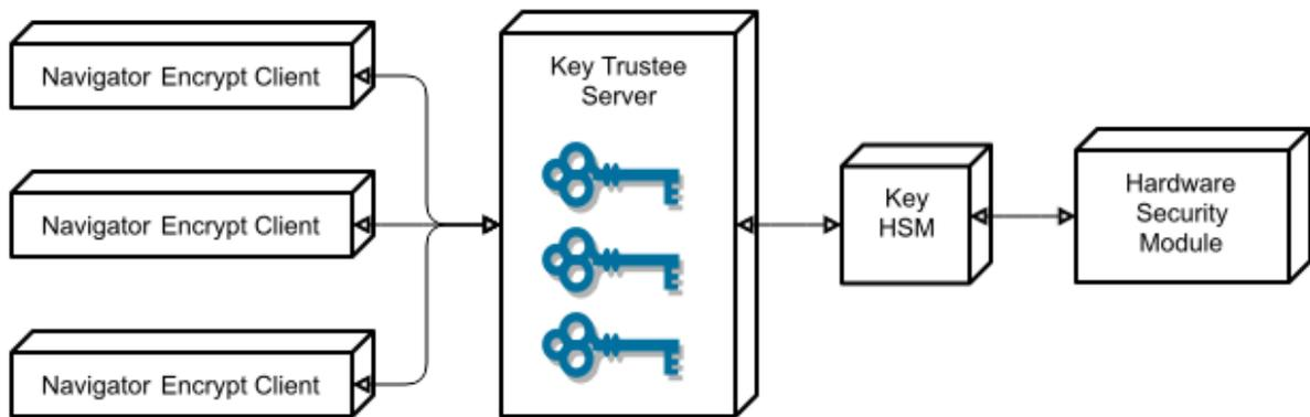
Key Trustee clients include Navigator Encrypt, Key Trustee KMS, and HSM KMS. Encryption keys are created by the client and stored in Key Trustee Server.
