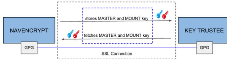
The master key is encrypted with a local GPG key. Before being stored in the Key Trustee Server database, it is encrypted again with the Key Trustee Server GPG key. When the master key is needed to perform a Navigator Encrypt operation, Key Trustee Server decrypts the stored key with its server GPG key and sends it back to the client (in this case, Navigator Encrypt), which decrypts the deposit with the local GPG key.
