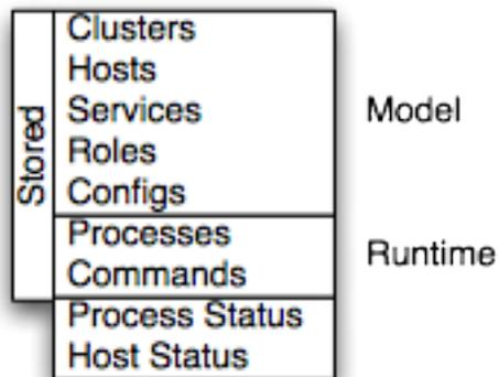
Cloudera Manager models CDH and managed services: their roles, configurations, and inter-dependencies. *Model state* captures what is supposed to run where, and with what configurations. For example, model state captures the fact that a cluster contains 17 hosts, each of which is supposed to run a DataNode. You interact with the model through the Cloudera Manager Admin Console configuration screens and API and operations such as "Add Service".
