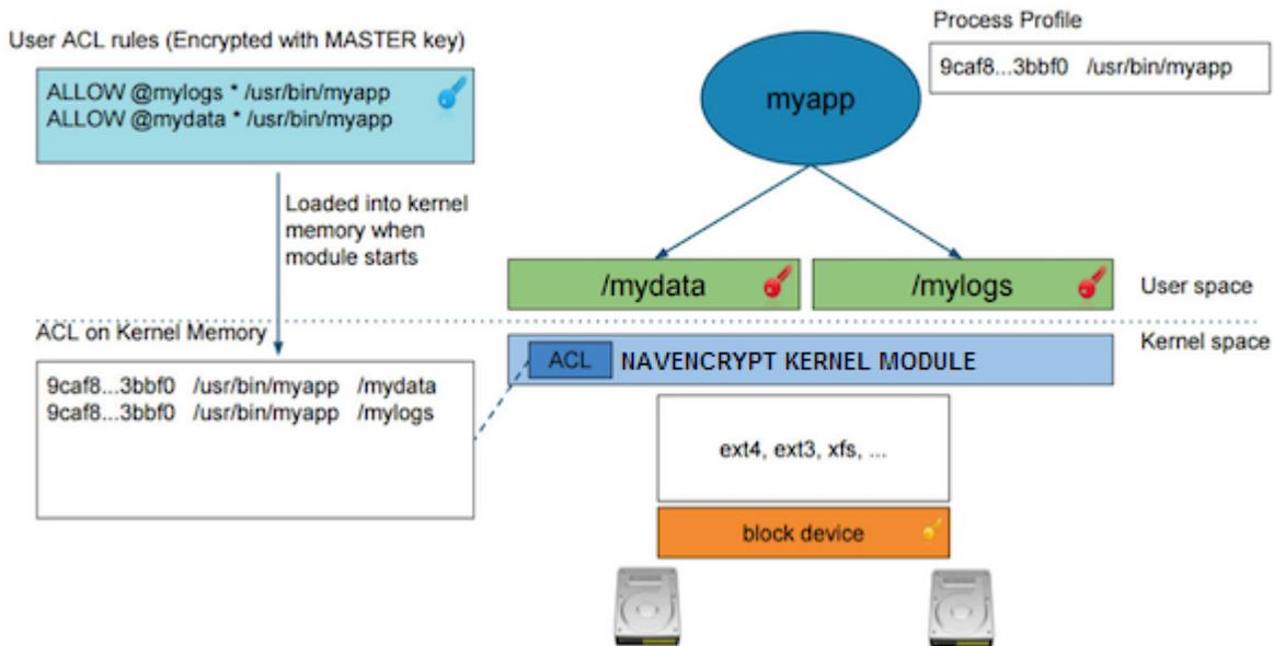
The user adds a rule to allow `/usr/bin/myapp` to access the encrypted data in the category `@mylogs`, and adds another rule to allow `/usr/bin/myapp` to access encrypted data in the category `@mydata`. These two rules are loaded into the `navencrypt-kernel-module` cache after restarting the kernel module.
