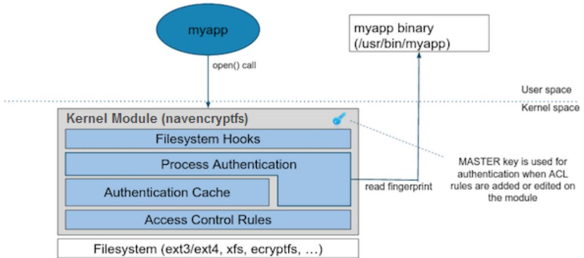
The kernel module calculates the process fingerprint. If the authentication cache already has the fingerprint, the process is allowed to access the data. If the fingerprint is not in the cache, the fingerprint is checked against the ACL. If the ACL grants access, the fingerprint is added to the authentication cache, and the process is permitted to access the data.
