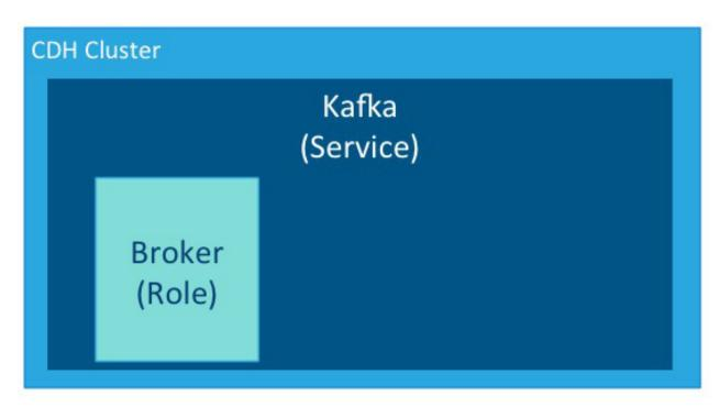
An instance is a deployed and configured software component. A cluster can include multiple roles and multiple instances of the same role. A service instance might be Kafka-1. Kafka-1 might host the role instances Broker-1, Broker-2, and Broker-3.
