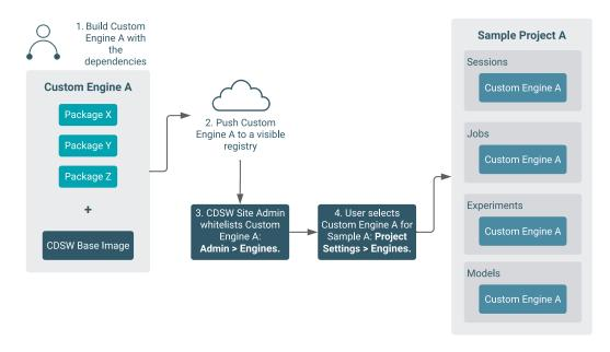
Directly installing a package to a project as described above might not always be feasible. For example, packages that require root access to be installed, or that must be installed to a path outside /home/cdsw (outside the project mount), cannot be installed directly from the workbench. For such circumstances, Cloudera recommends you extend the base Cloudera Machine Learning engine image to build a customized image with all the required packages installed to it.
