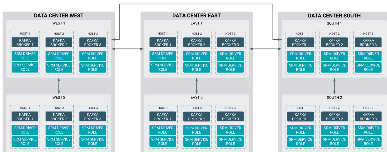
Figure 2: Cross Data Center Replication of Multiple Clusters
